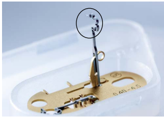
Application of the laser: To determine the correct settings the surgical laser is tested on the Thermo-Dummy and adjusted accordingly.
